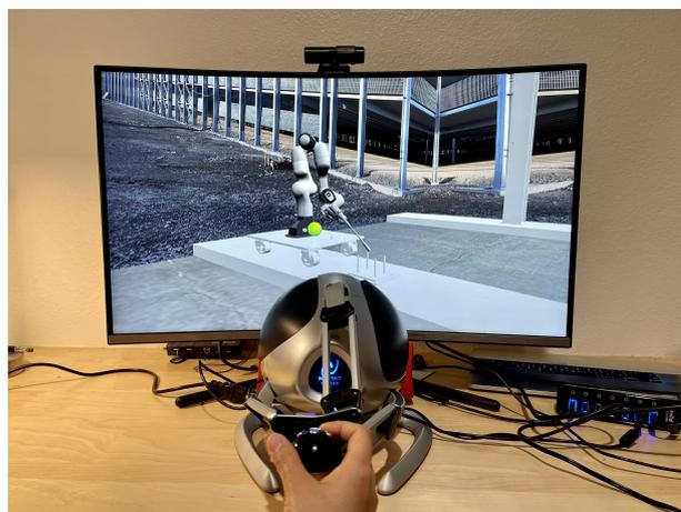
Figure 1: Robotic solution to a welding task combining robot autonomy and haptic human intervention. Video of task execution: [video](#). Source code can be found here: [Project GitHub](#).
